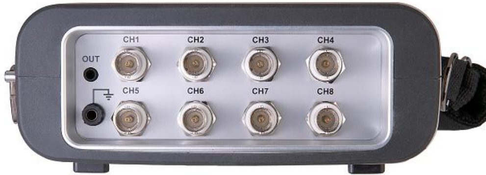
Figure 1 CoCo-90 contains 4 or 8 BNC input connectors and an output source channel.
