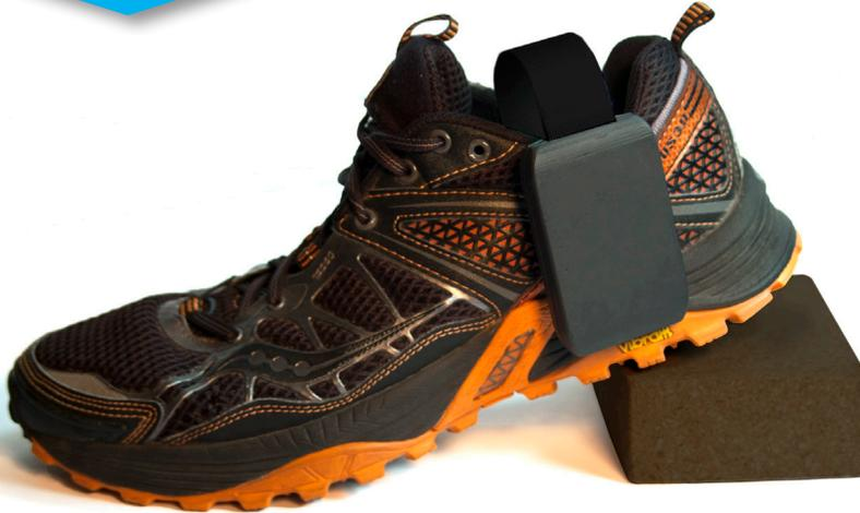
The Tactilus® wireless foot insole sensor system inserted into a shoe
